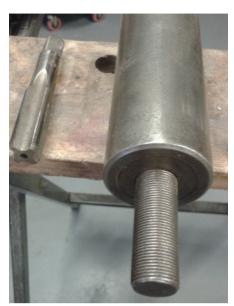
Plate 2 - Mounting bar showing the threaded stud for attaching the Planer
