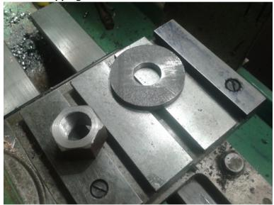
Plate 4 - Completed mounting nut and 5.7mm thick washer
