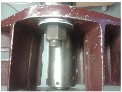
Plate 5 - Completed mounting nut and 5.7mm thick washer
